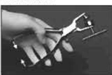
3. Compress handles together in order to create pressure on the bone material.
