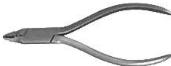
20-217 Young Wire bending and loop forming pliers ● 0.36 mm to 0.71 mm (.014" to .028") ■ Max. 0.56 mm x 0.71 mm (.022" x .028")
